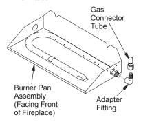
Figure 7 - Connecting Gas to Appliance
